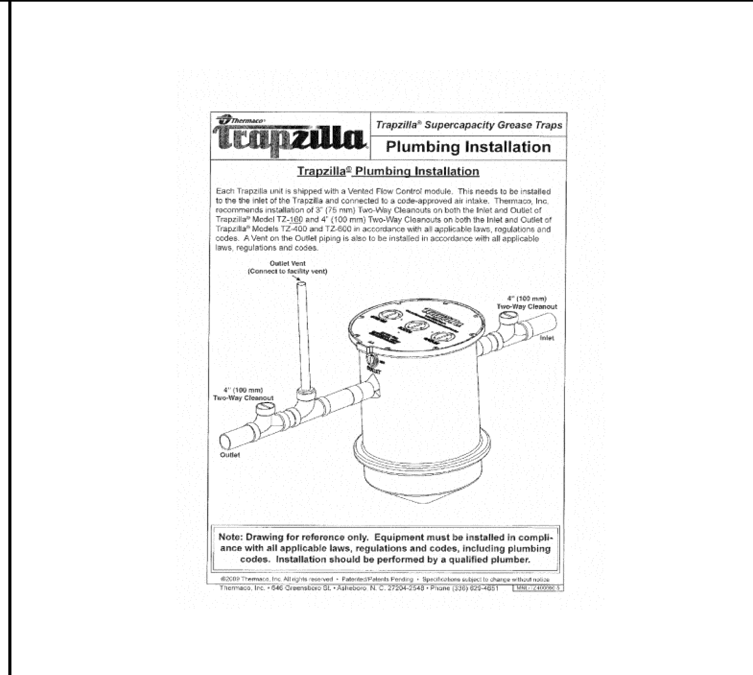
2 GREASE TRAP DETAIL
